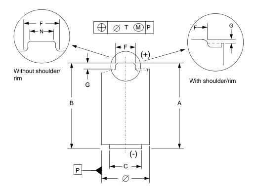
Figure 2A – Round battery (protruding negative)
