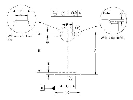
Figure 2B – Round battery (recessed negative)
