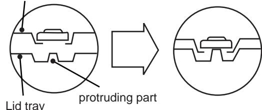
\*Lay a tray lid flat and place a tray containing batteries on top of it: batteries are pushed up by protrusions of the lid tray so that they can be easily picked up with fingers.
