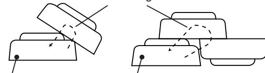
\*Contact of batteries with each other forms discharge circuits, thus the batteries are drained.
