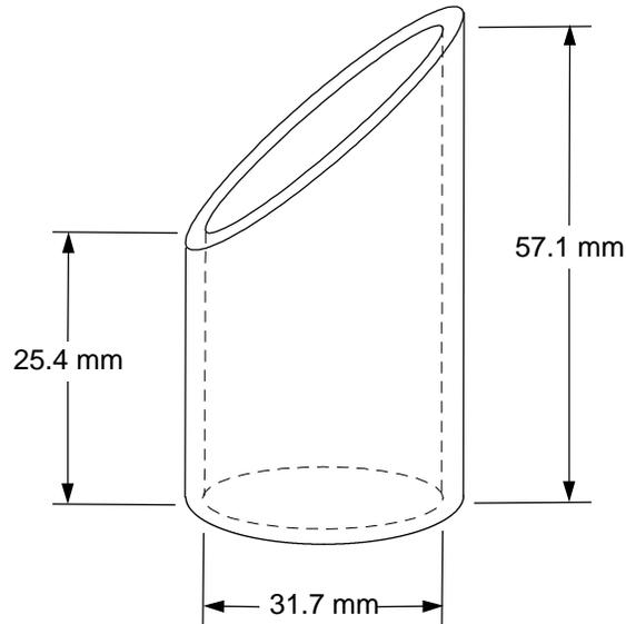
**Figure 1 – Small cell or battery gauge
